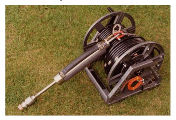
REVERSIBLE SPRING LOADED HAMMER, 100 FOOT SINGLE THREE-IN-ONE CABLE, ZERO-TIME TRIGGER SOURCE INPUT TO SEISMOGRAPH, CABLE REEL, AIR PUMP AND GAUGE, ALUMINUM SHIPPING CASE, SPARE PARTS KIT
